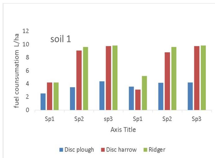
**Figure 4. Effect of different forward speeds and tractors power on fuel Consumption (l/hr) at two different soils**
